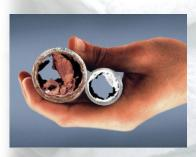
Calcium Scale is a hard thick coating or cover-ing of calcium carbonate (CaCO<sub>3</sub>) that forms on heating elements and on the pipes and hardware of plumbing systems. As the calcium rich water enters
